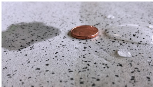
Left: unprotected - water penetrates the surface
